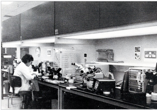
Figure 8. A laminar flow hood keeps the work area clean for the handling and bonding of beam lead devices onto circuits.
